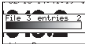
Progress bar shown during file refresh after a time without power.
