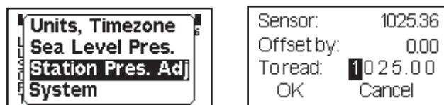
Main Menu / Set-up / Station Pressure Adjust menu.
